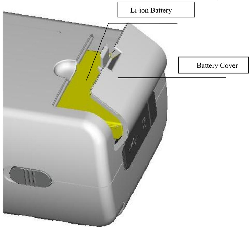
Figure 4 Battery Installation
