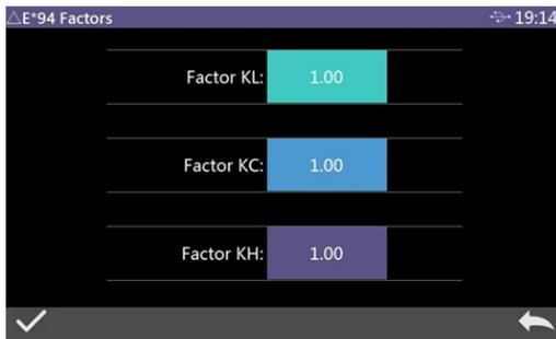
Figure 43  $\Delta E^*_{94}$  Factor setting interface
