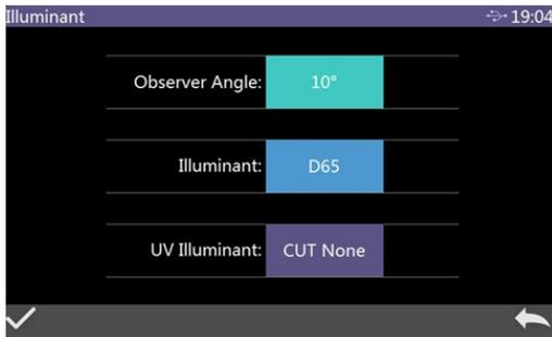
Figure 13 Light Source Setting Interface
